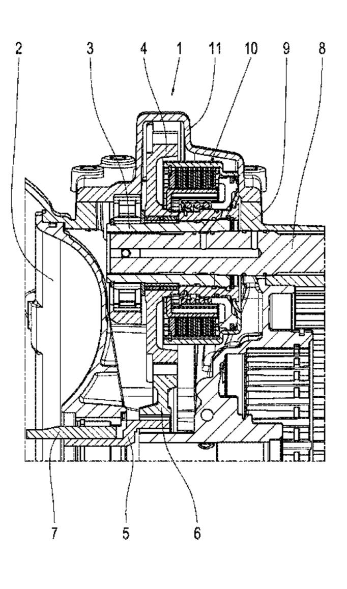
can be connected to an additional unit to be driven, and having a switching element. The power take-off element is arranged on a power take-off shaft and can be connected to the power take-off shaft via the switching element, which is arranged to act between power take-off shaft and the power take-off element.
