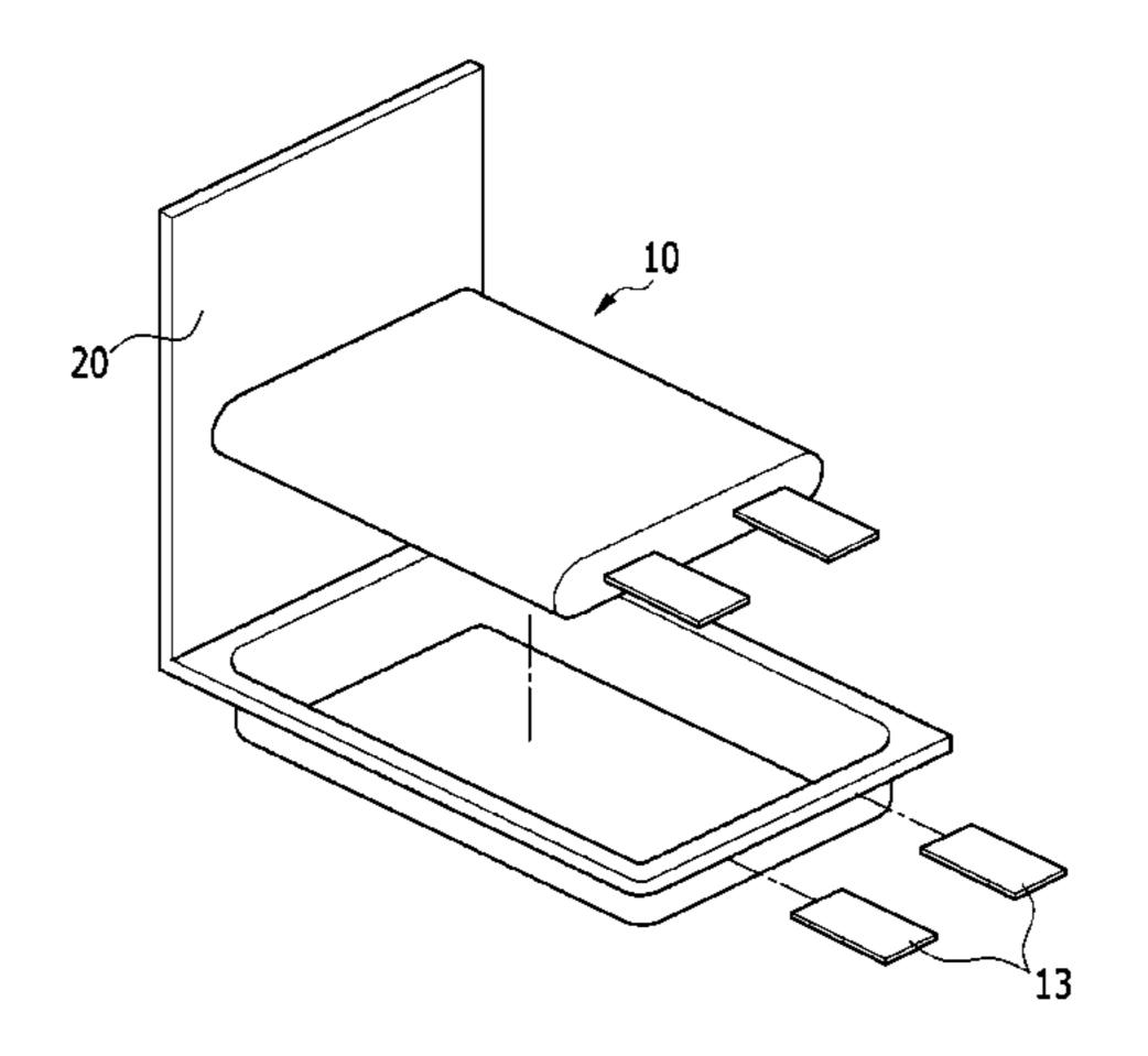
binations thereof. The rechargeable lithium battery has improved cycle-life and high temperature storage characteristics.
