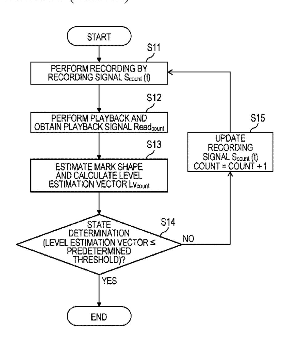
of the recording signal, and a level of the recording signal is adjusted.
