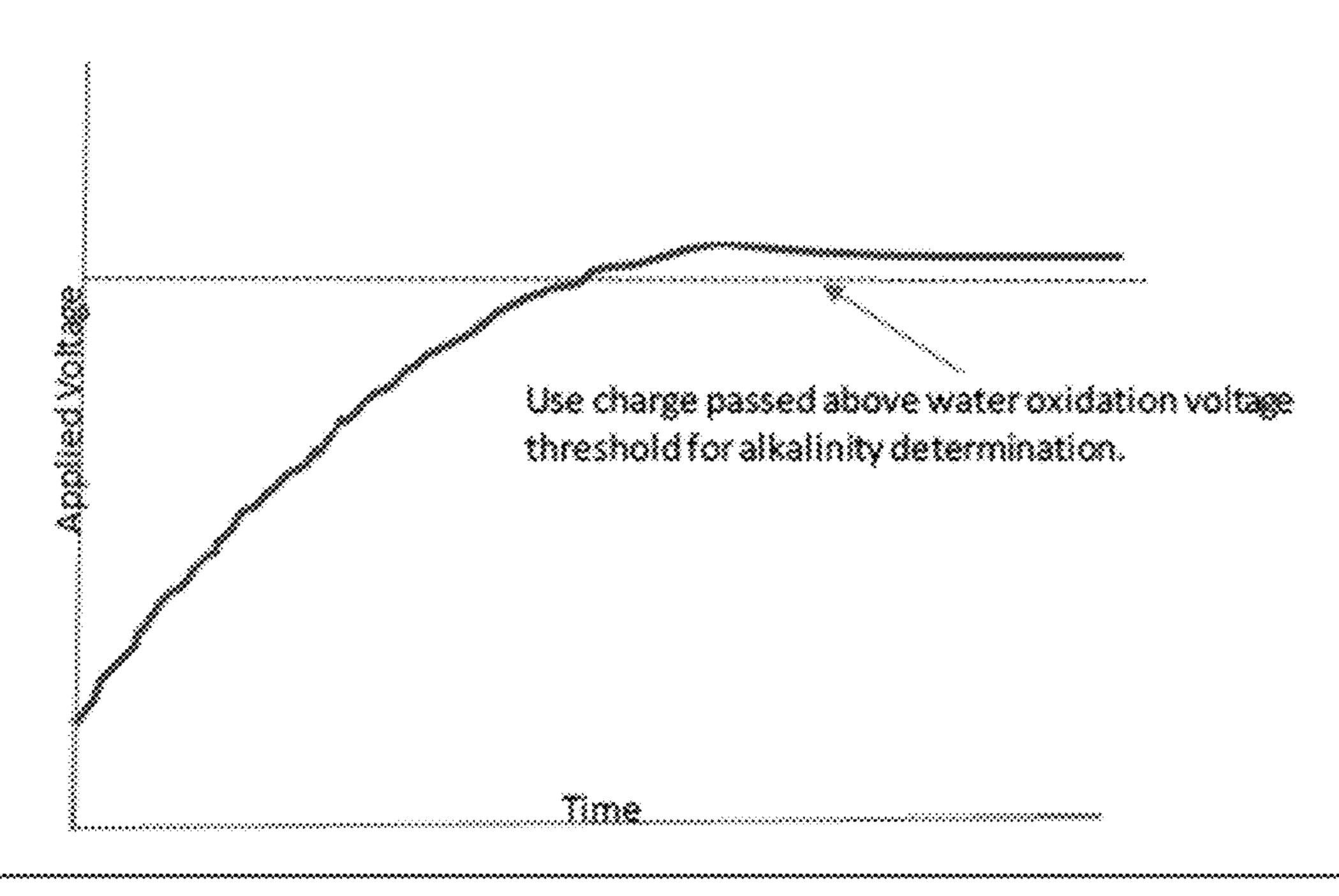
Voltage-time profile that serves as a diagnostic tool to determine and mitigate the effects of interference during a reagent less alkalinity measurement using electrochemical methods
