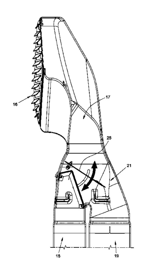
and third channel; and an air adjusting device to adjust the air temperature in the third channel and comprising a shutter coupled to the first channel and/or to the second channel and/or to the connection element; and a control device controlling a position of the shutter to adjust the temperature of the air entering the third channel.
