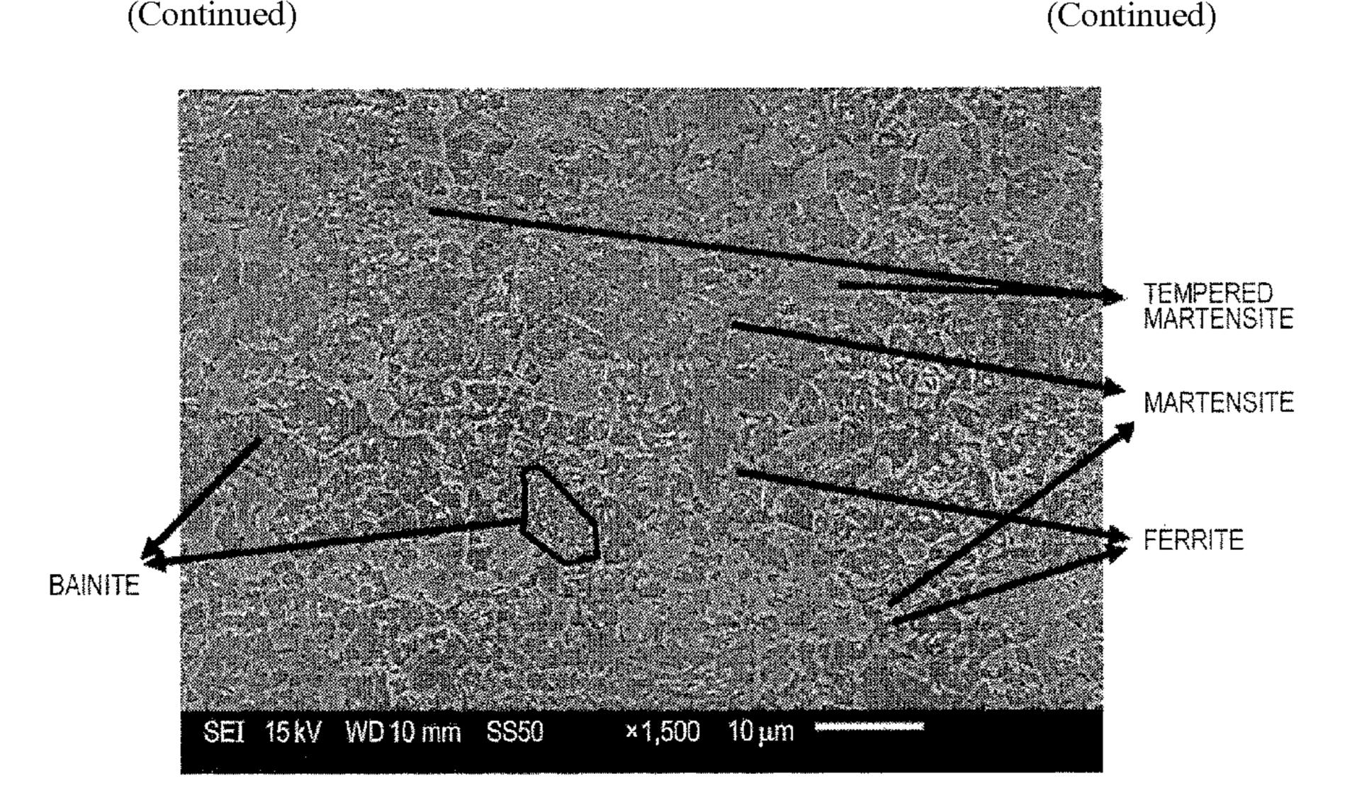
layer formed on the steel sheet having a coating weight of 20 g/m<sup>2</sup> to 120 g/m<sup>2</sup> per side, in which a yield strength ratio is 65% or more, a tensile strength is 950 MPa or more, and Mn oxides are contained in the galvanized layer in an amount of 0.015 g/m<sup>2</sup> to 0.050 g/m<sup>2</sup>.
