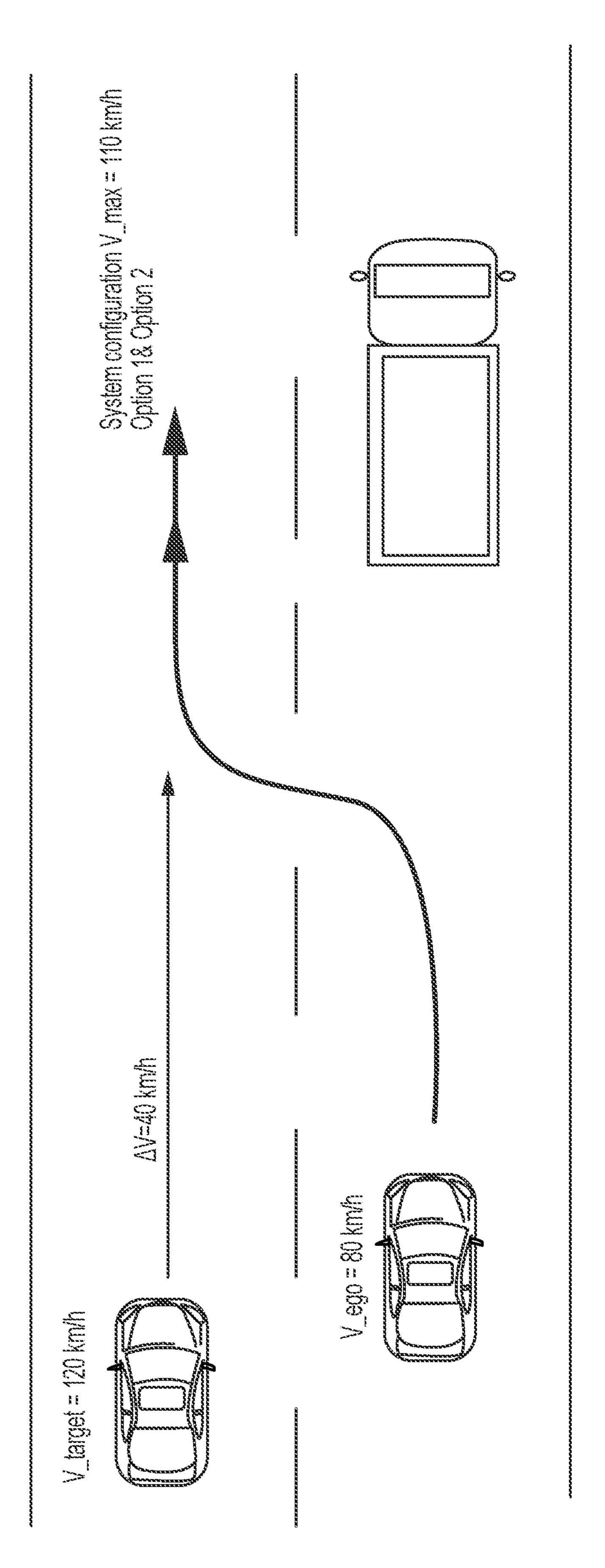
Option 1. Accelerate to adapt with V\_target and execute lane change fully automatically Option 1. Accelerate to adapt with V\_target and execute lane change maneuver
