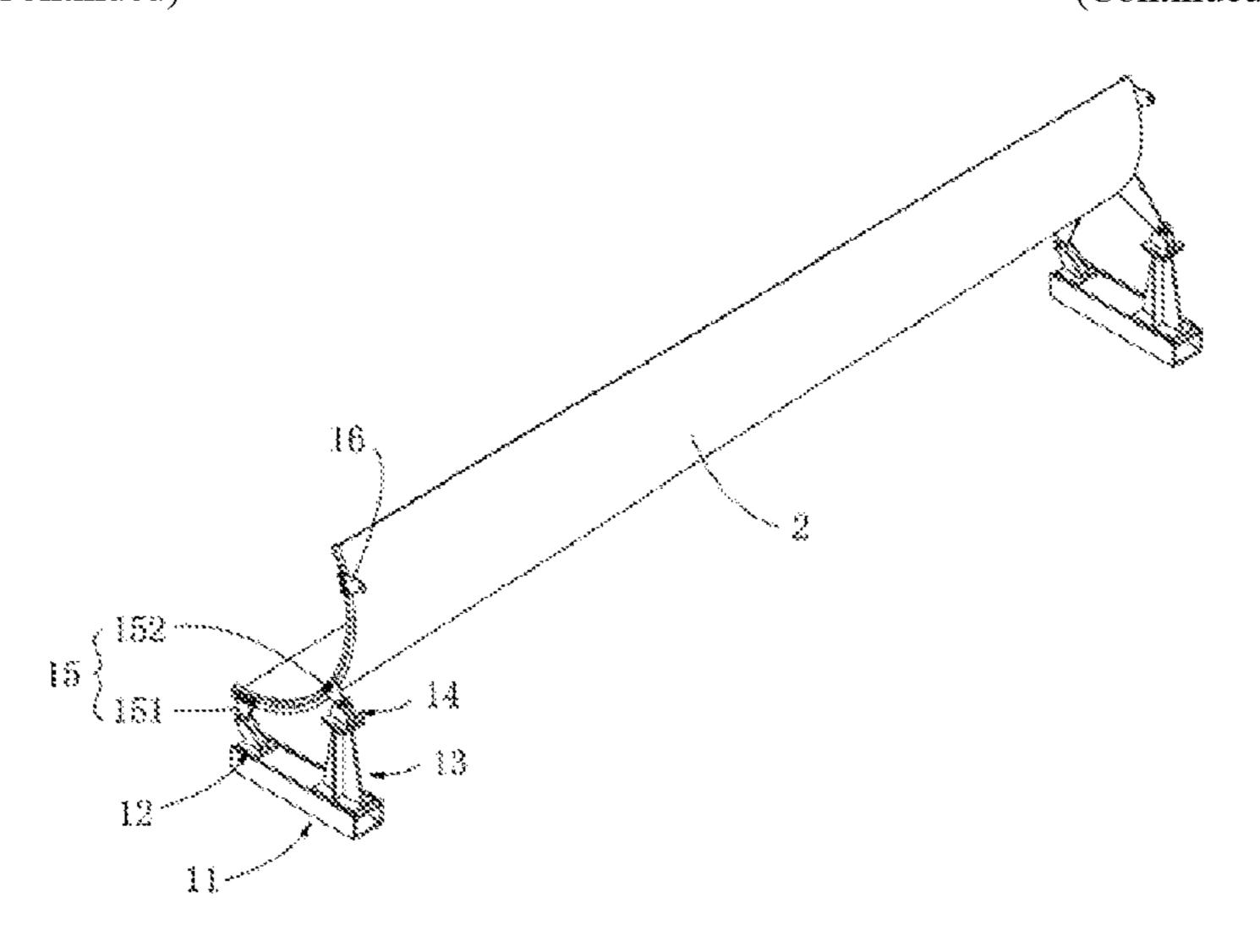
member on the second direction and connected to the fixing member; wherein in the second direction, a height of the support member is higher than that of the first hinge member, the first hinge member is adapted to rotatably connect with the tower tube segment and serve as a rotation fulcrum of the tower tube segment, and the support member is adapted to support the tower tube segment to maintain a position of the tower tube segment relative to the first hinge member.
