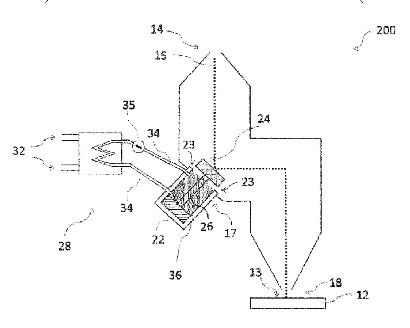
(26), wherein the cooling device (28) has at least one primary circuit (30) through which a first cooling fluid can flow without contact with the actuator (26). Furthermore, a set of parts for a machining apparatus for laser machining a workpiece (12) and a method of laser machining a workpiece (12) using such machining apparatus are also provided.
