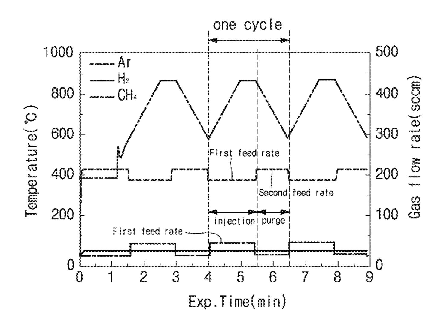
one cycle of temperature control and the cycle is repeated for a predetermined process time.
