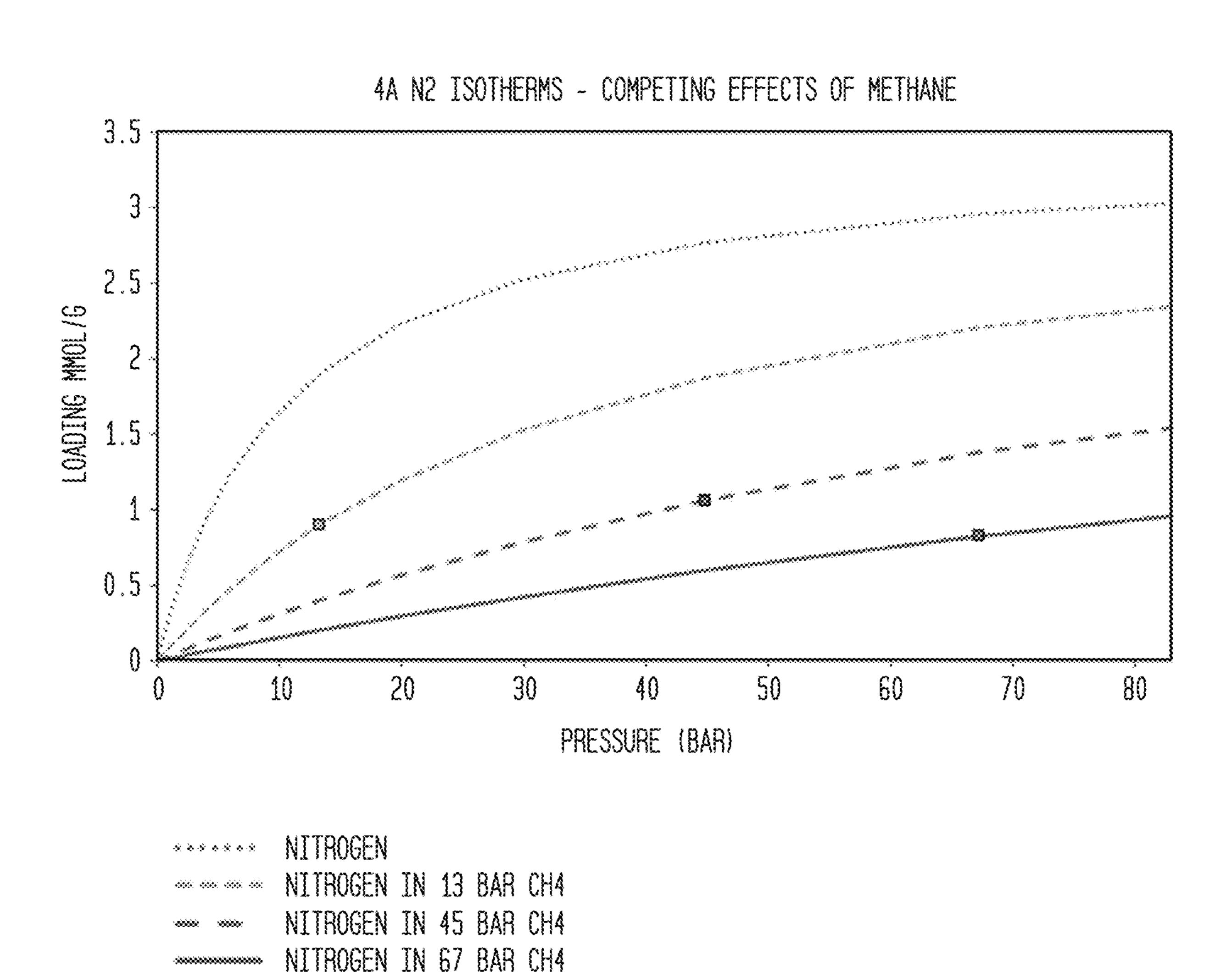
MAX CAPACITY POINT FOR 13 BAR
