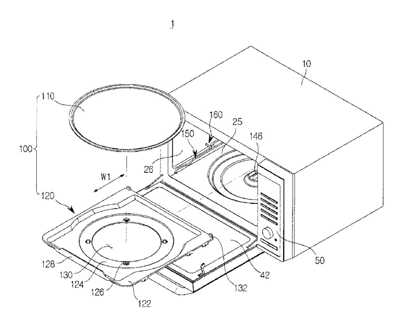
sible to easily switch between the rotatable state of the tray and the state of sliding movement of the tray.
