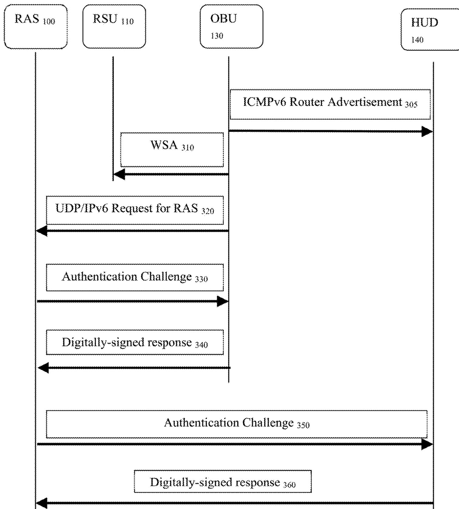
Figure 4 Propagation of WSMP notifications to the Heads-Up Display
