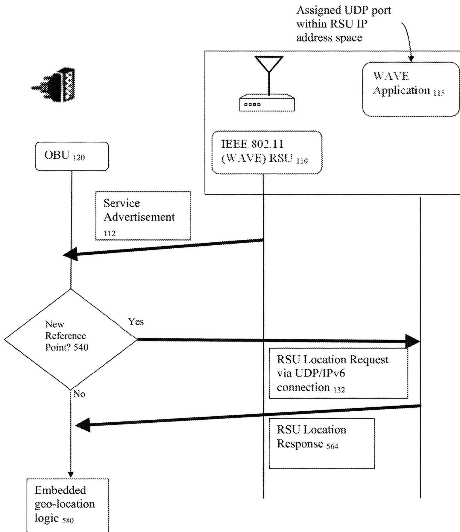
Figure 14a Geo-positioning with WAVE-Enabled Smart Phone
