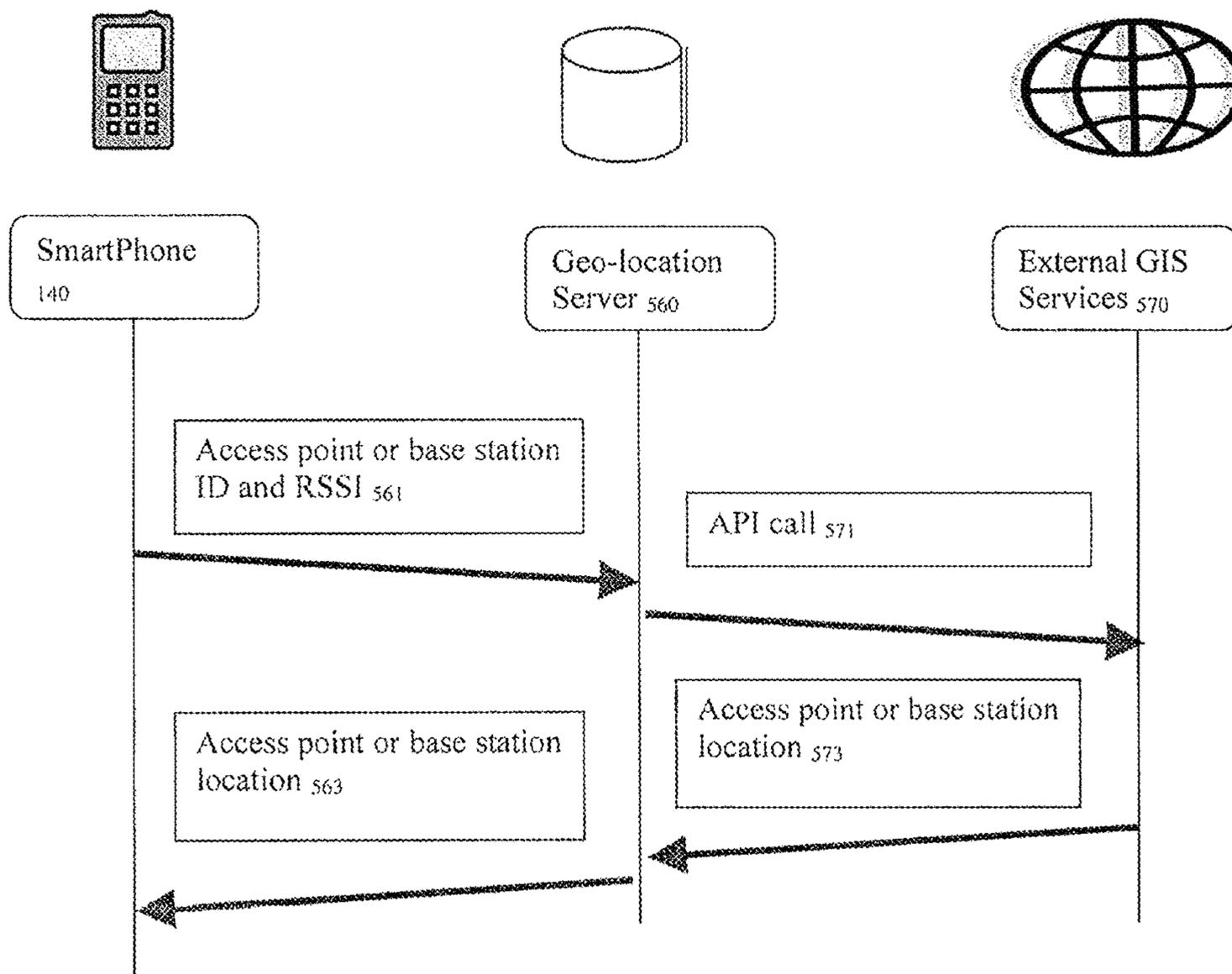
Figure 11 Embedded Geo-location Logic
