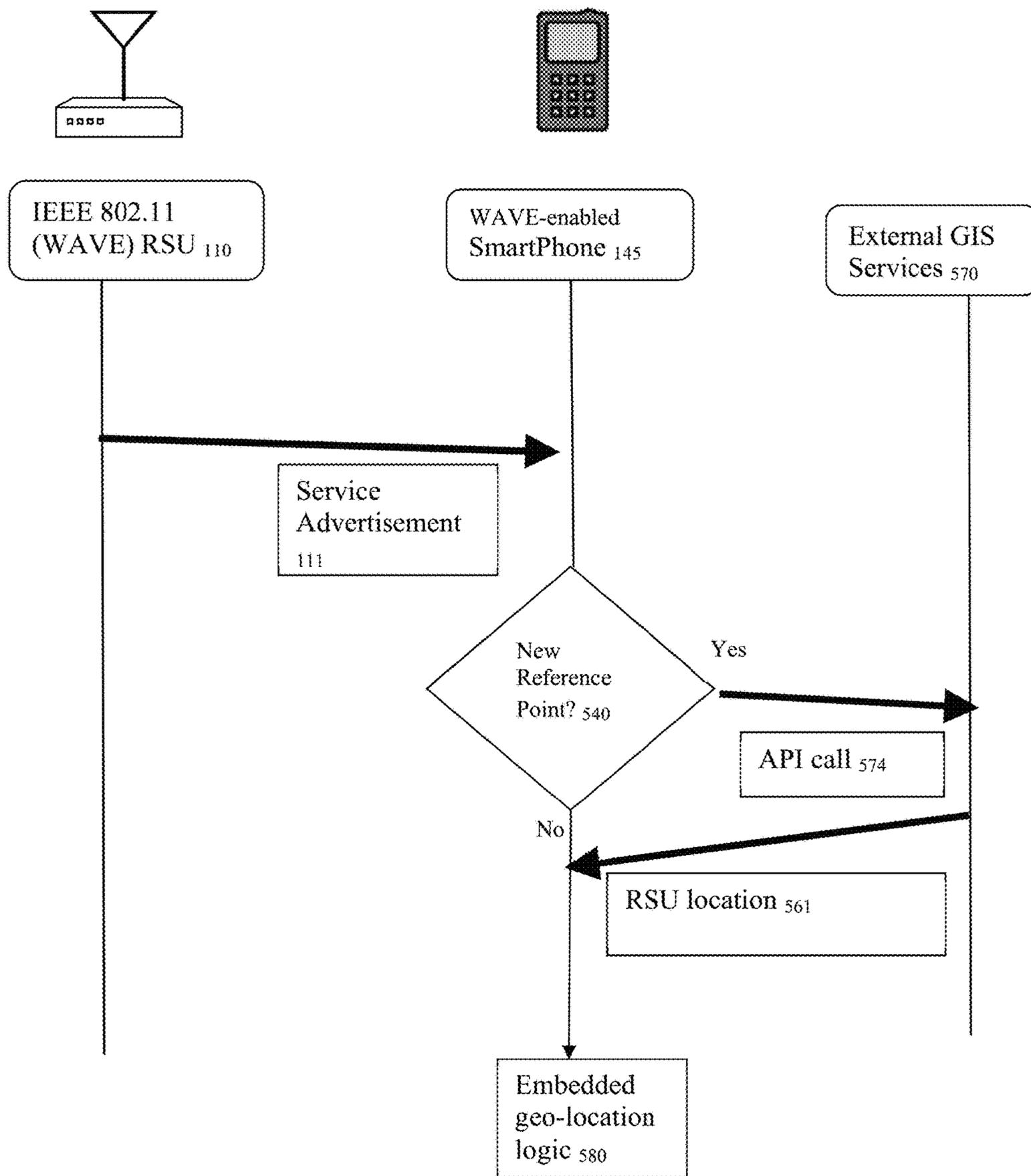
Figure 14b Geo-positioning with 2 WAVE RSUs
