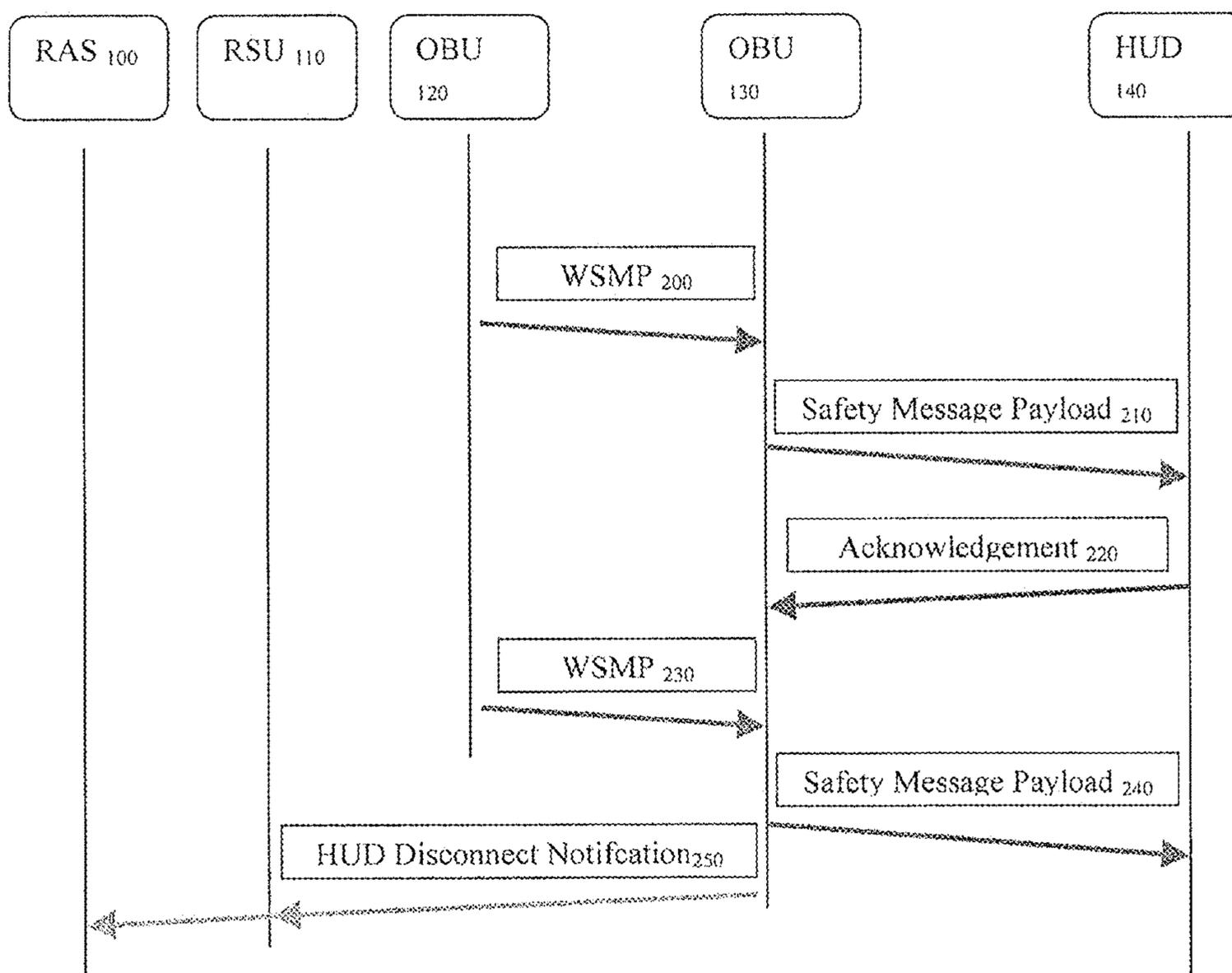
Figure 5 ATP Communications with a WAVE-Enabled OBU
