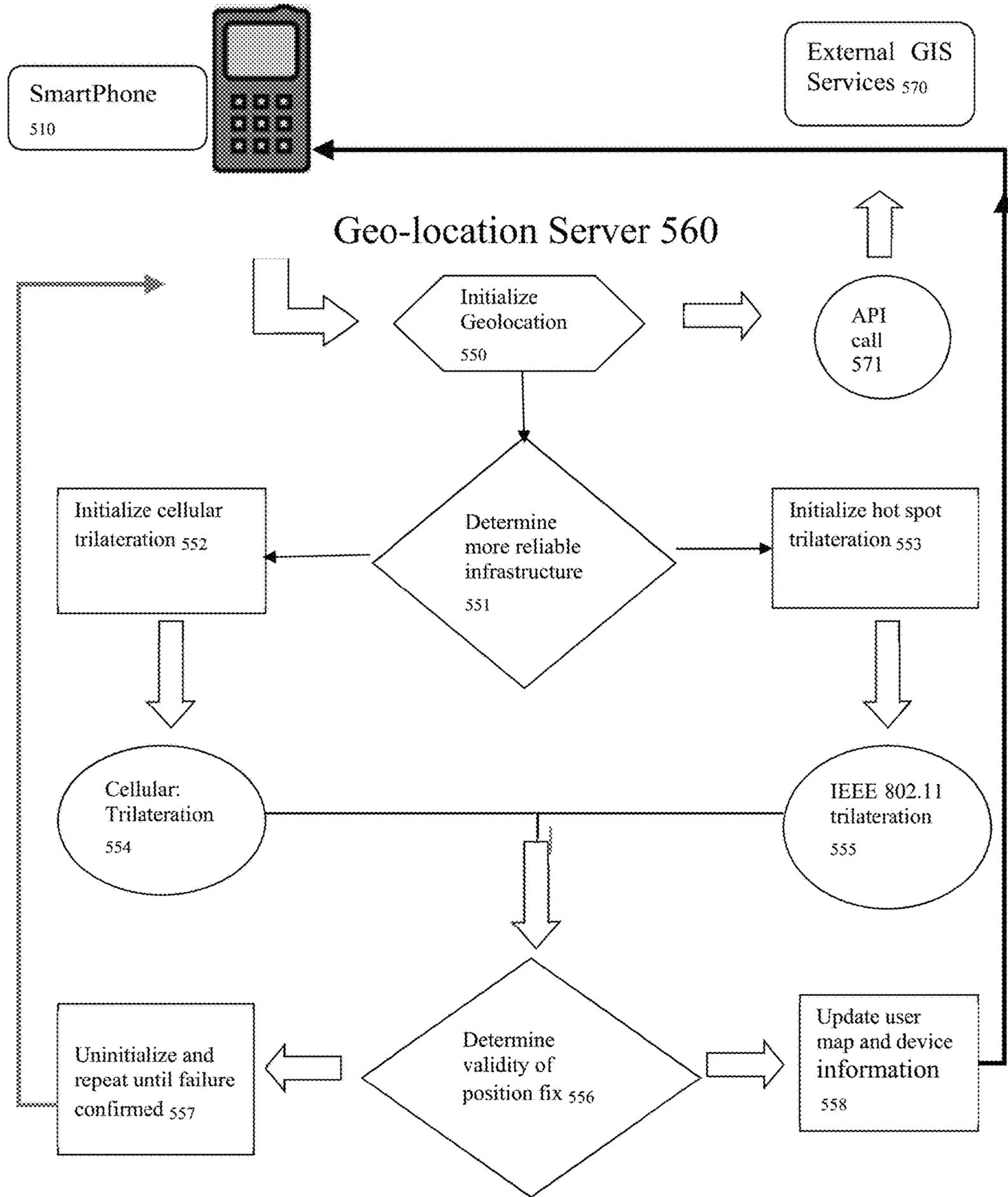
Figure 10 Geo-location of New Access Point or Base Station
