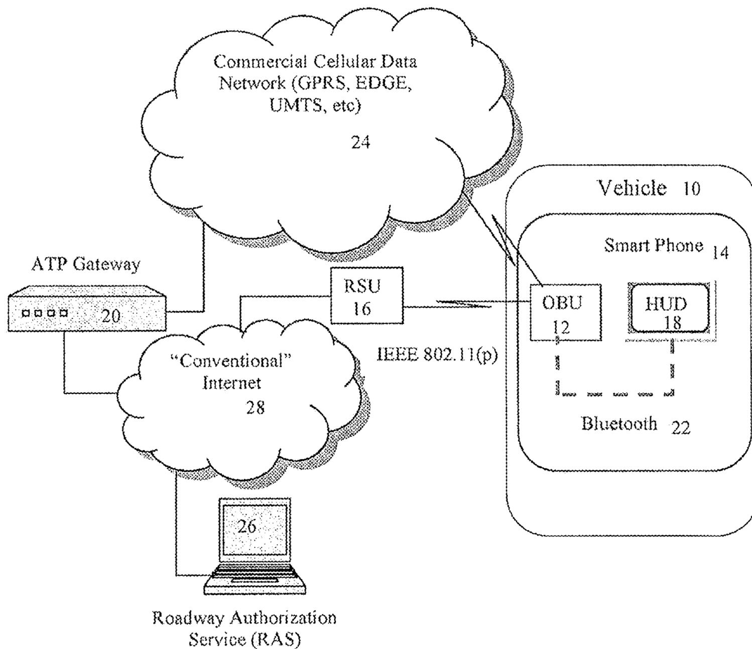
Figure 3 OBU and Heads-Up Display Authentication
