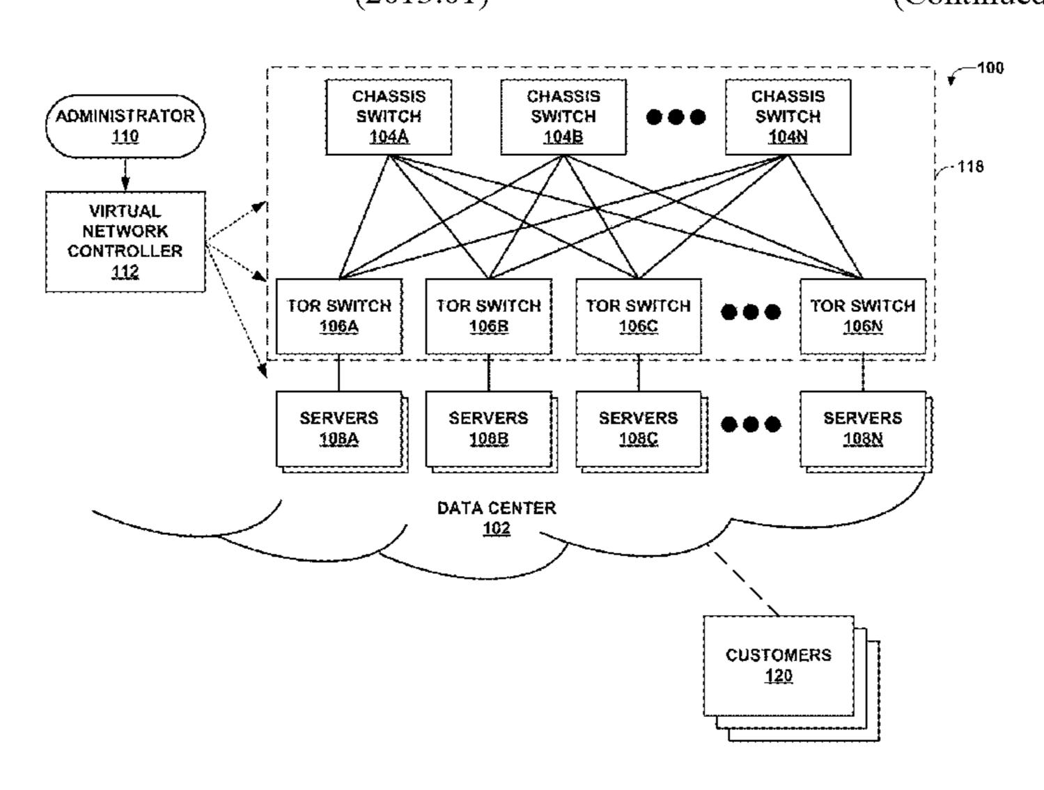
switch fabric for application to communications through the logical router interconnect.
