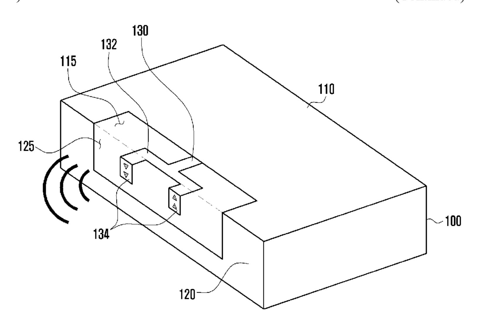
angle with the first plate in contact with the first plate, and has a second opening surface on one side surface so as to extend the first opening surface, and a power supply unit which has one surface electrically connected to the first plate and is disposed on the first opening surface or the second opening surface.
