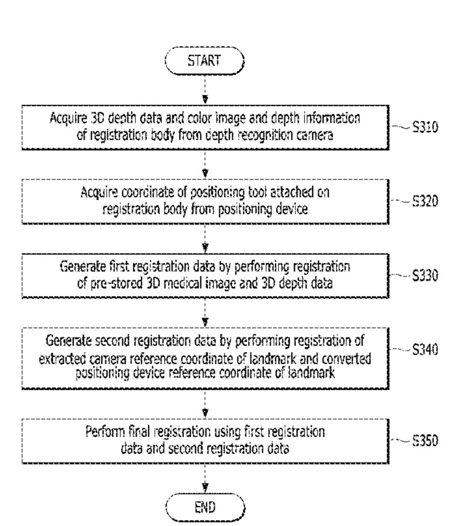
registration body and converting pre-stored relative position information of the landmark with reference to the three-dimensional coordinates of the positioning tool, to perform registration of camera reference three-dimensional coordinates of the landmark and the converted position information thereof; and a third registration unit performing final registration by using results of registration performed by the first registration unit and the second registration unit.
