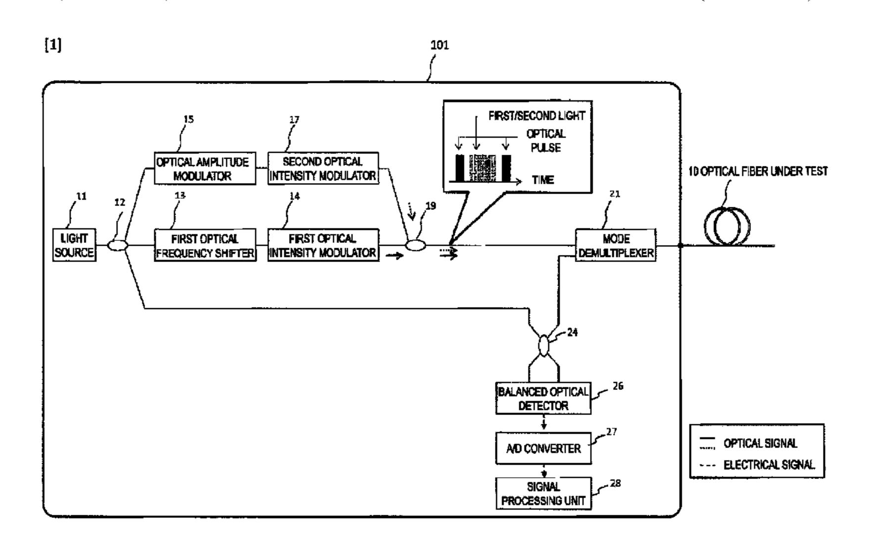
the local oscillation light generated by the local oscillation light generation unit and photoelectrically convert the multiplexed light into an electrical signal, and an arithmetic processing unit configured to calculate a time-intensity distribution of the electrical signal obtained by the light reception unit photoelectrically converting the backscattered light in the LP11 mode.
