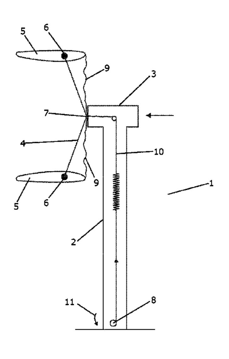
pivot angle in the case of an emergency, the stop mechanism comprising a release mechanism (8, 12, 14) and at least one wire (9, 10) interconnecting the release mechanism (8, 12, 14) and each of the wind turbine blades (5). Activation of the release mechanism (8, 12, 14) causes an abrupt change in a pulling force applied to the wind turbine blades (5) by the wire(s) (9, 10), the change in pulling force causes the wind turbine blades (5) to move immediately to the safe pivot angle.
