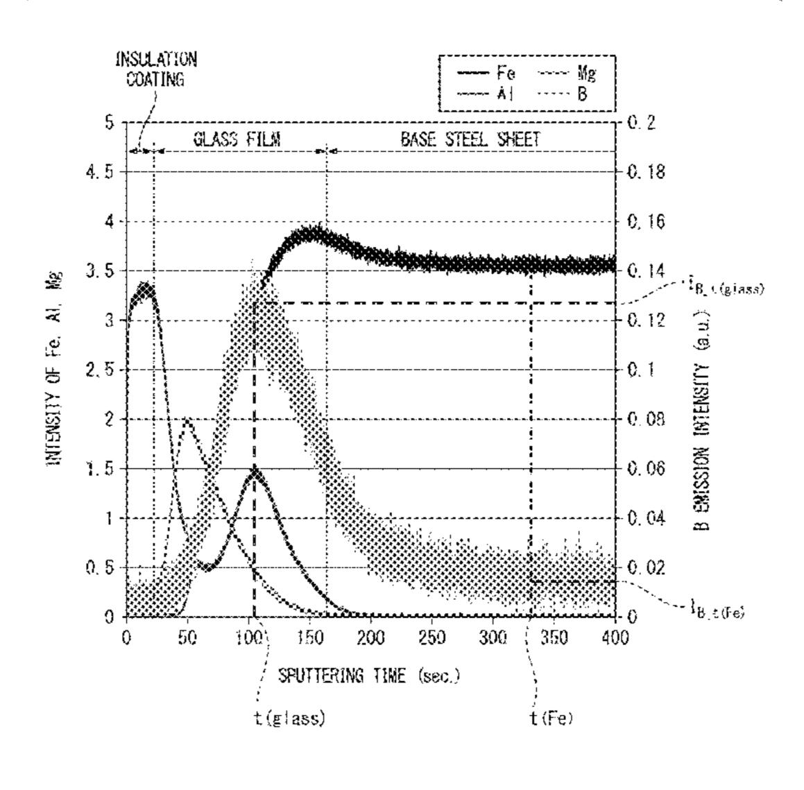
B emission intensity obtained inside the glass film is more than a B emission intensity obtained inside the base steel sheet, when a B emission intensity is measured from a surface of the insulation coating by a glow discharge emission spectroscopy.
