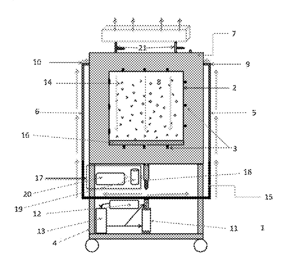
chamber. Such a system can in particular be used to test the integrity of a container and/or the antimicrobial activity of a product of interest.
