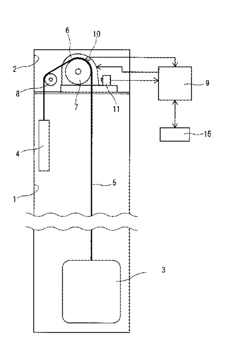
threshold value is predicted for each measuring point, and the earliest time is displayed as a rope replacement time (S12\_S14).
