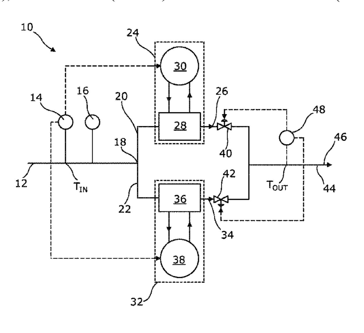
(22). The conditioning assembly (10) still further includes an output conduit (44) to receive the first and second propellant streams (26, 34). The relative proportion of the first and second propellant streams (26, 34) merging in the output conduit (44) is controlled to regulate the temperature of a merged constant pressure propellant feed (46) exiting from the output conduit (44).
