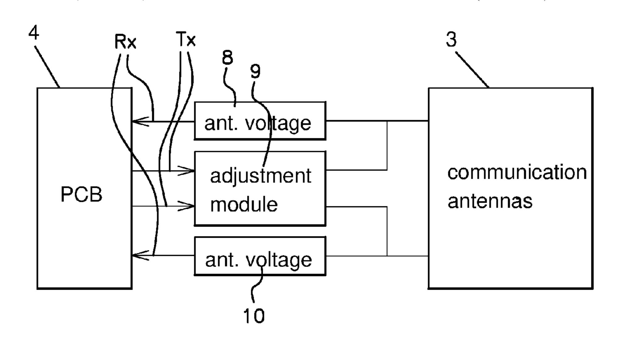
reception unit with an electronic control unit having a unit for activating the function. The communication antenna is movable relative to the printed circuit board under the action of the deformation of the component, the measuring unit then detecting a voltage variation across the terminals of the communication antenna.
