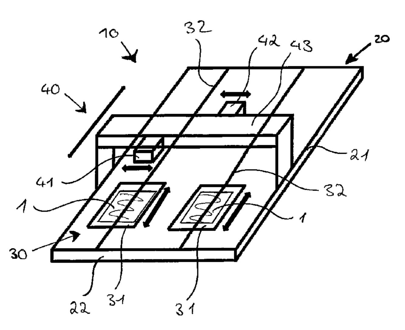
print head unit and at least one second print head unit of the printing device are independently moved over the width of the holding base body relative to each other along a guide device and print the at least one print object with a printed image.
