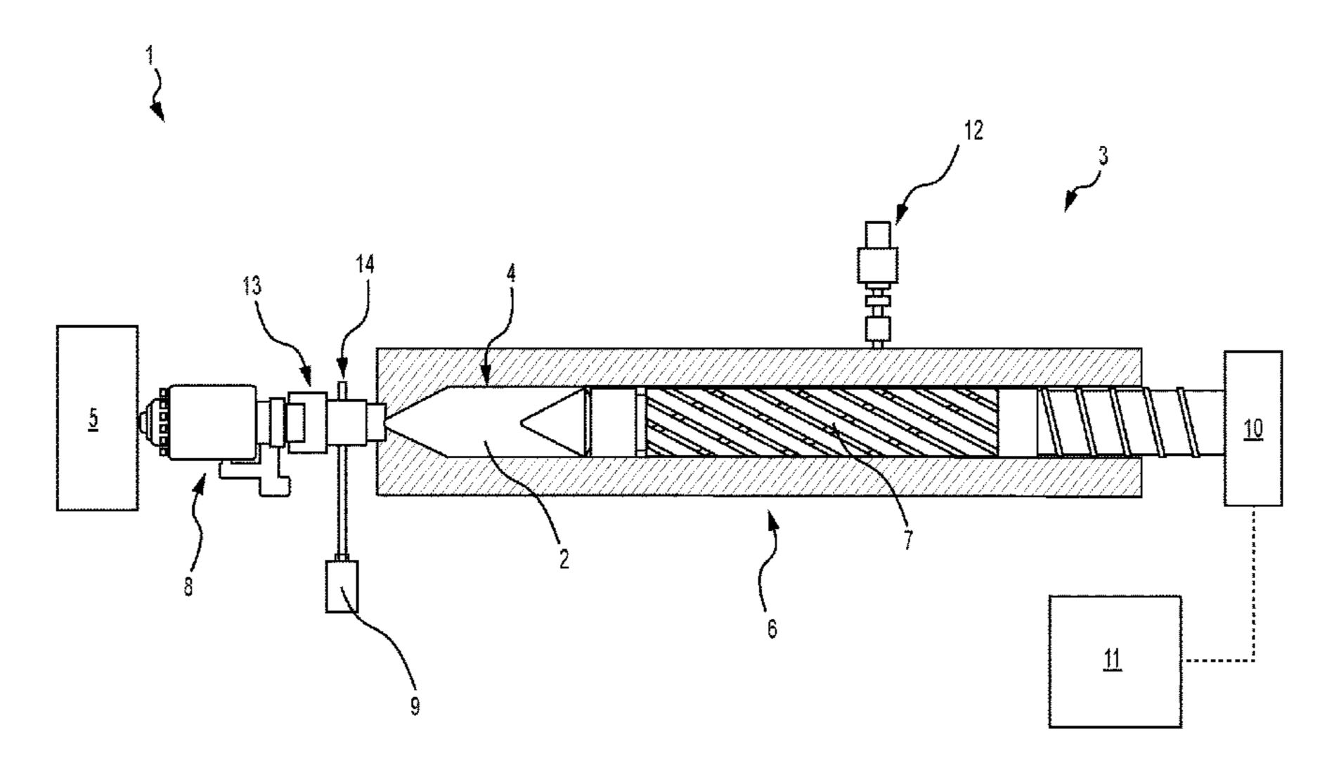
gas in the plastic melt is determined from the at least one compression parameter.
