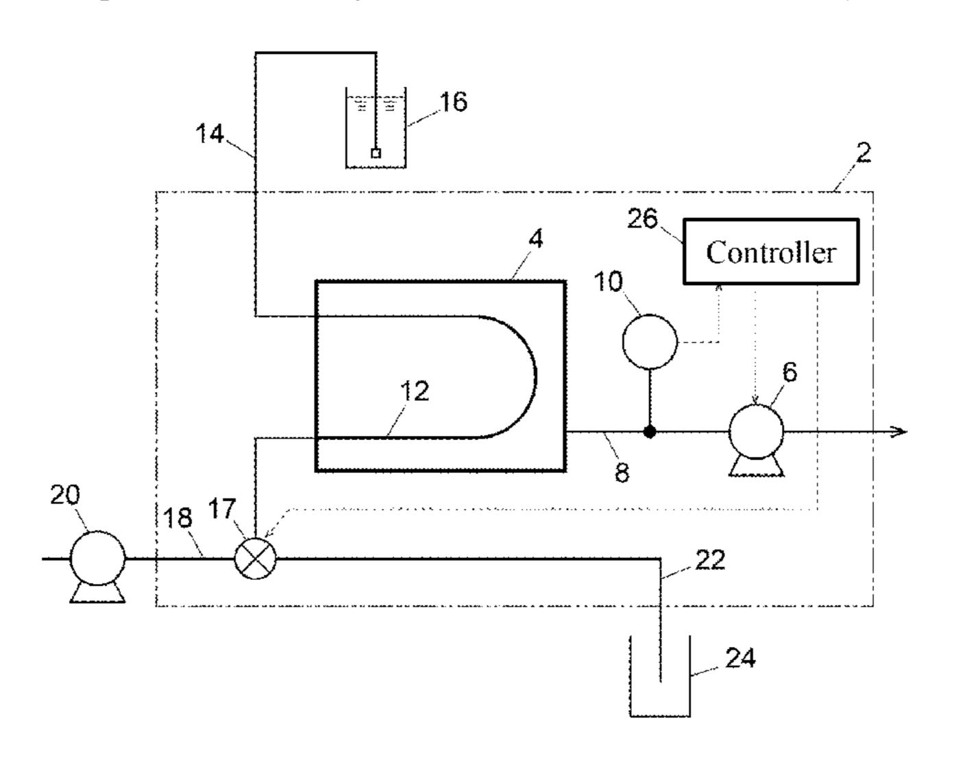
phase by the liquid feeding pump is stopped to drain the mobile phase in the degassing flow path through the drain flow path.
