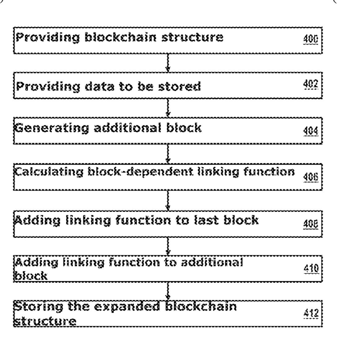
last block and of the additional block, using the data stored in the last block and the data to be stored in the additional block; and associating the combined check value with a block-independent, linking process-specific function. The method further includes adding the first block-dependent linking function to the last block and to the additional block.
