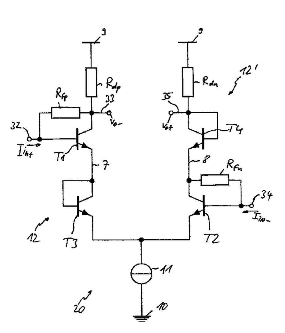
voltage of the first amplifier part is proportional to the input current of the first amplifier part and an output voltage of the second amplifier part is proportional to an input current of the second amplifier part.
