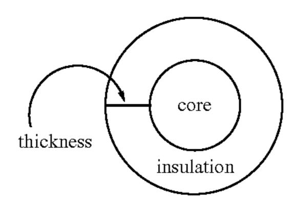
ISO 6722 test either at 125° C., or 150° C. or preferably both. There are three categories of cable which can be subjected to the ISO test 6722: thick wall, thin wall or ultra-thin wall. They are categorised based on the insulation thickness in relation to the conductor diameter and size. The 40 thinner the wall, the more challenging it is to pass the ageing standard.
