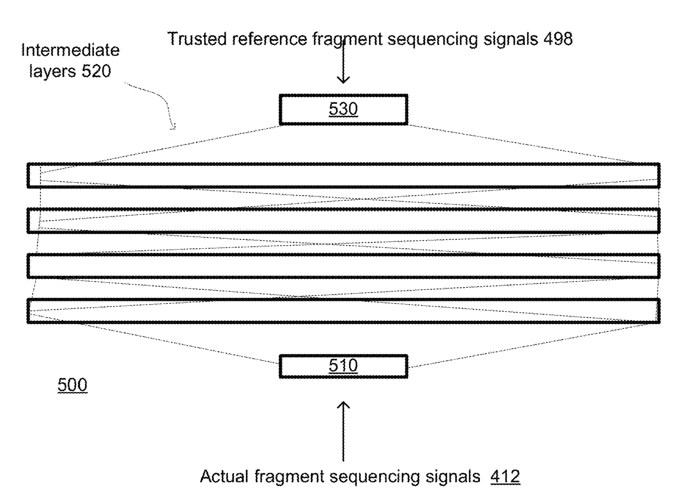
Generating, using a first machine learning process, a first mapping between actual reference sequencing signals to trusted reference sequencing signals. The actual reference sequencing signals and the trusted reference sequencing signals and trusted reference sequencing signals represent parts of a reference genome of a first genus. 610
