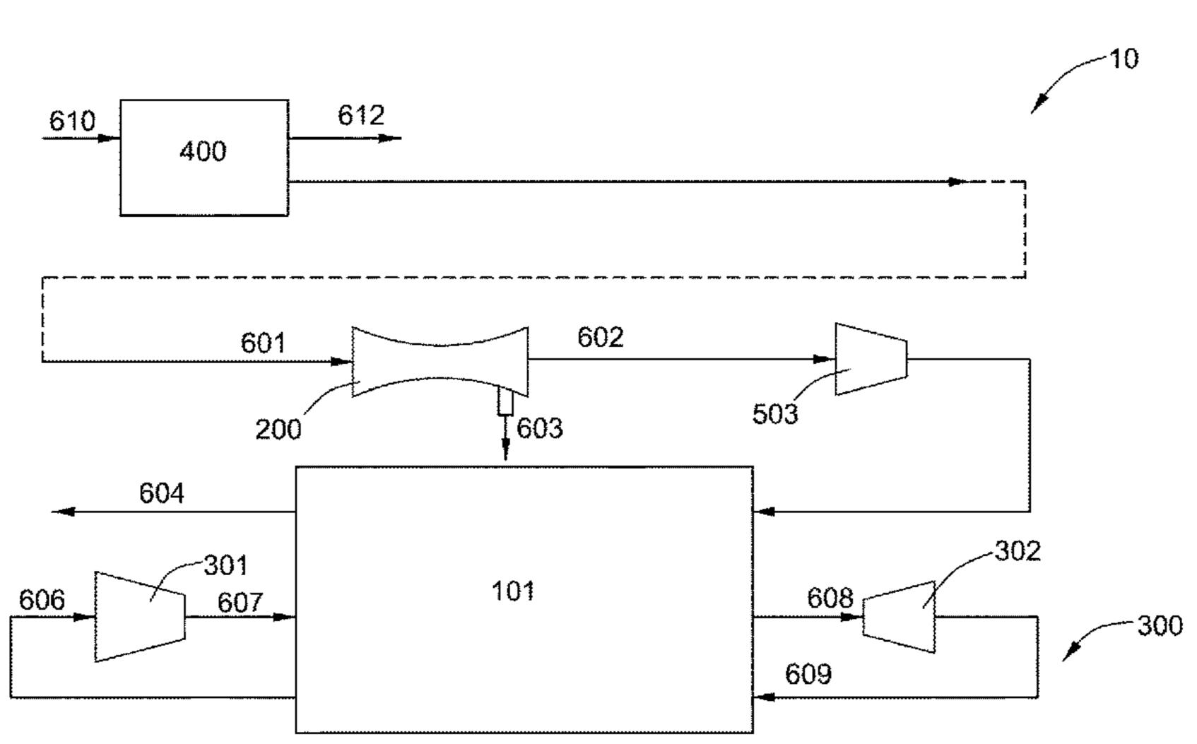
gaseous natural gas stream to obtain a second gaseous natural gas stream, and a cold box for receiving the cold stream of refrigerant and the second gaseous natural gas stream and cooling the second gaseous natural gas stream to obtain a liquefied natural gas by heat exchanging between the second gaseous natural gas stream and the cold stream of refrigerant.
