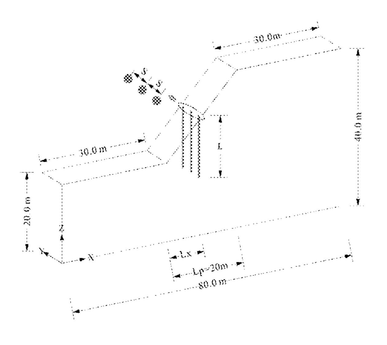
the comprehensive optimization value, and determining whether the optimal anti-slide pile reinforcement scheme meets the optimization objective; and carrying out slope reinforcement according to the optimal anti-slide pile reinforcement scheme if yes. A multi-objective comprehensive optimization model including an optimization index system and comprehensive weights of optimization indexes is established.
