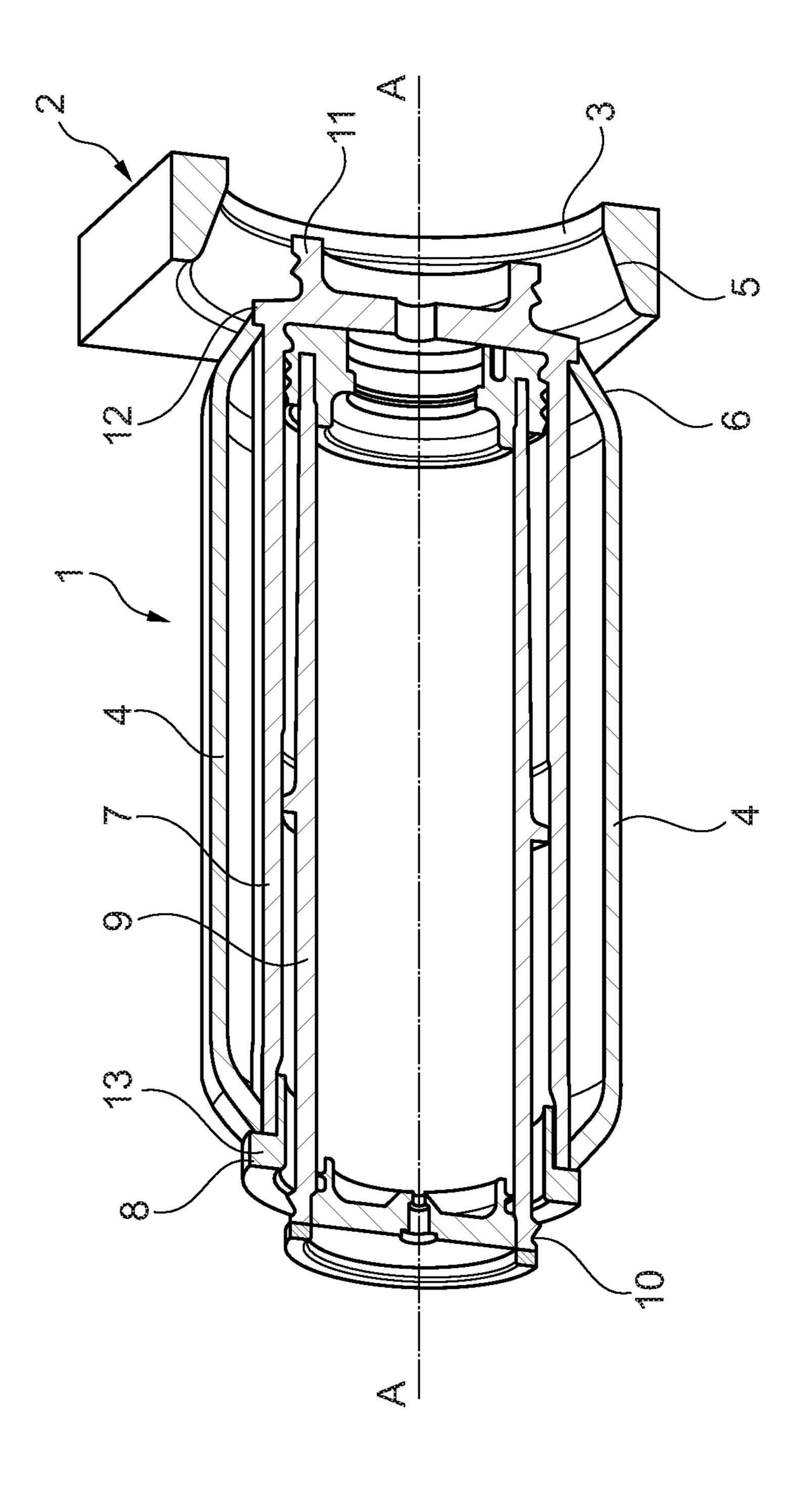
ENERGY DISSIPATING DEVICE SUITABLE TO BE USED AS PART OF A CONNECTION DEVICE THAT CONNECTS A FIRST CAR OF A MULTI-CAR VEHICLE WITH A SECOND CAR OF A MULTI-CAR VEHICLE AND METHOD FOR DISSIPATING ENERGY IN A **CONNECTION DEVICE**
