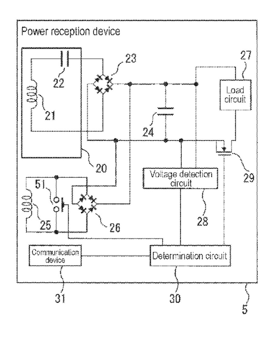
according to a voltage generated in the sub-coil to the smoothing capacitor in response to a voltage obtained by rectifying a voltage generated in the sub-coil being higher than a voltage between both terminals of the smoothing capacitor.
