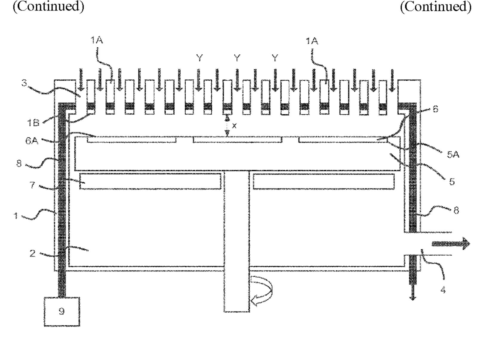
until it is proximate the substrate surface thus minimizing decomposition or other reaction of the precursor before it is proximate the substrate surface. The separation between the precursor inlet and the substrate is less than 100 mm.
