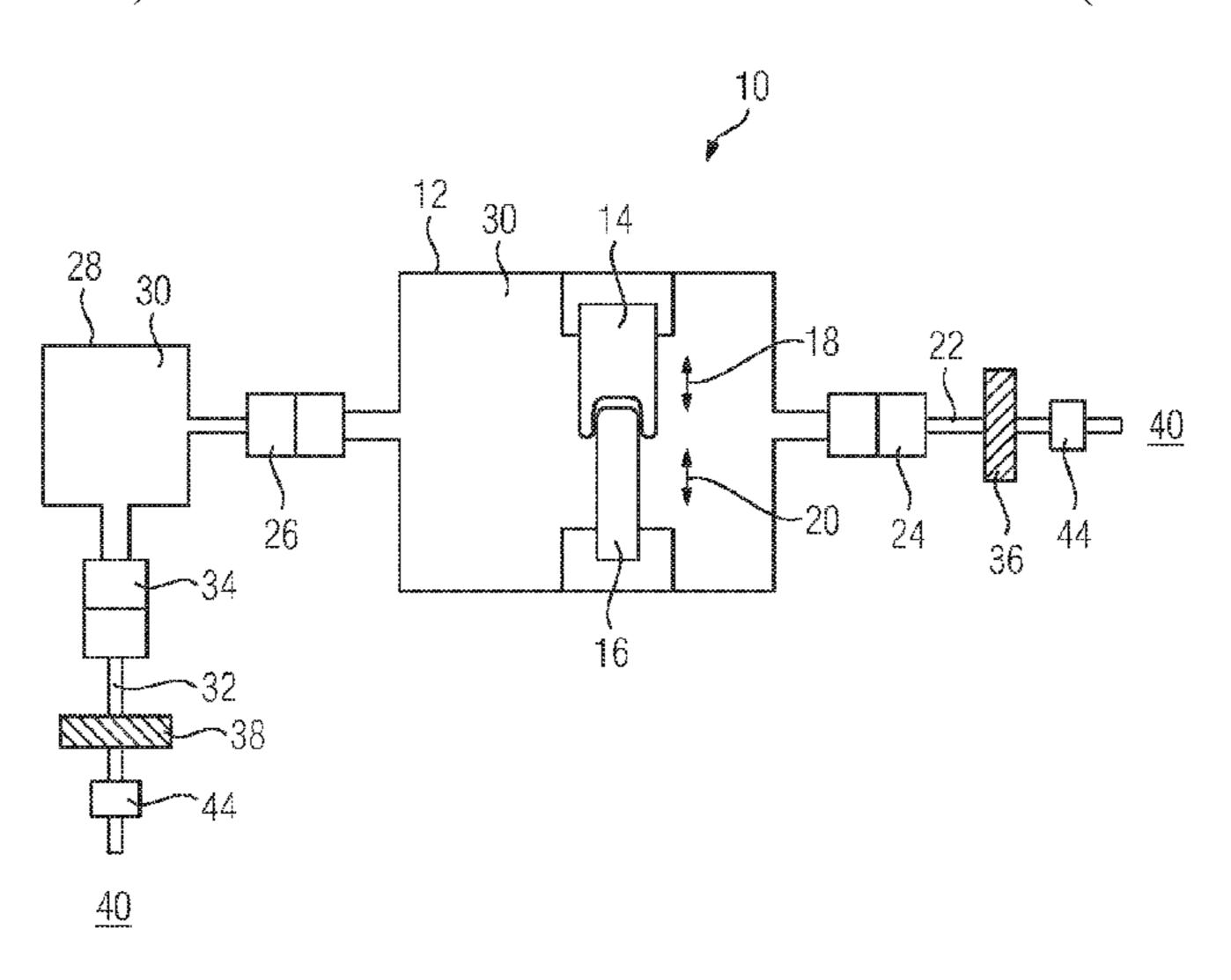
action. A fluid insulation medium is also provided, which is arranged in the switching chamber or in a storage volume which can be connected to the switching chamber. The switching chamber or the storage volume has an outlet for letting out the fluid insulation medium. A filter is provided at or adjacent to the outlet, the filter configured to filter gaseous components of the insulation medium, or the reaction products thereof, conducted through the outlet.
