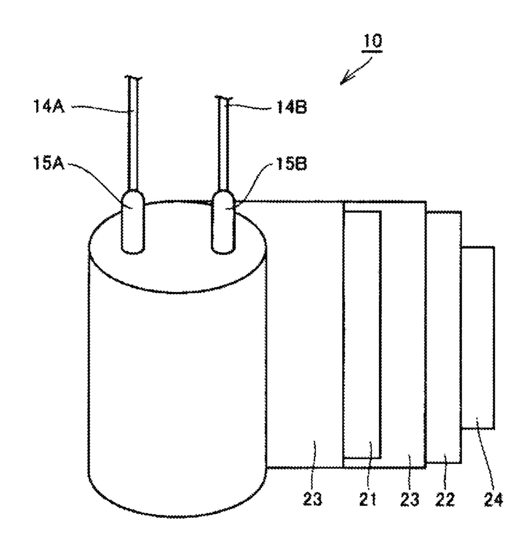
ELECTROLYTIC CAPACITOR COMPRISING AN ANODE BODY, A CATHODE BODY AND A CONDUCTIVE POLYMER AND A LIQUID COMPONENT DISPOSED BETWEEN THE ANODE BODY AND THE CATHODE BODY
