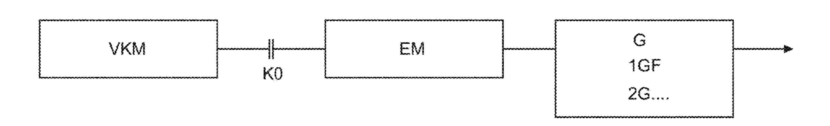
generator operation of the electric machine for energy recovery. The overrun torque thereby substantially corresponds to an overrun torque of a free-wheel-free configuration of the free-wheel-connected low forward gear.
