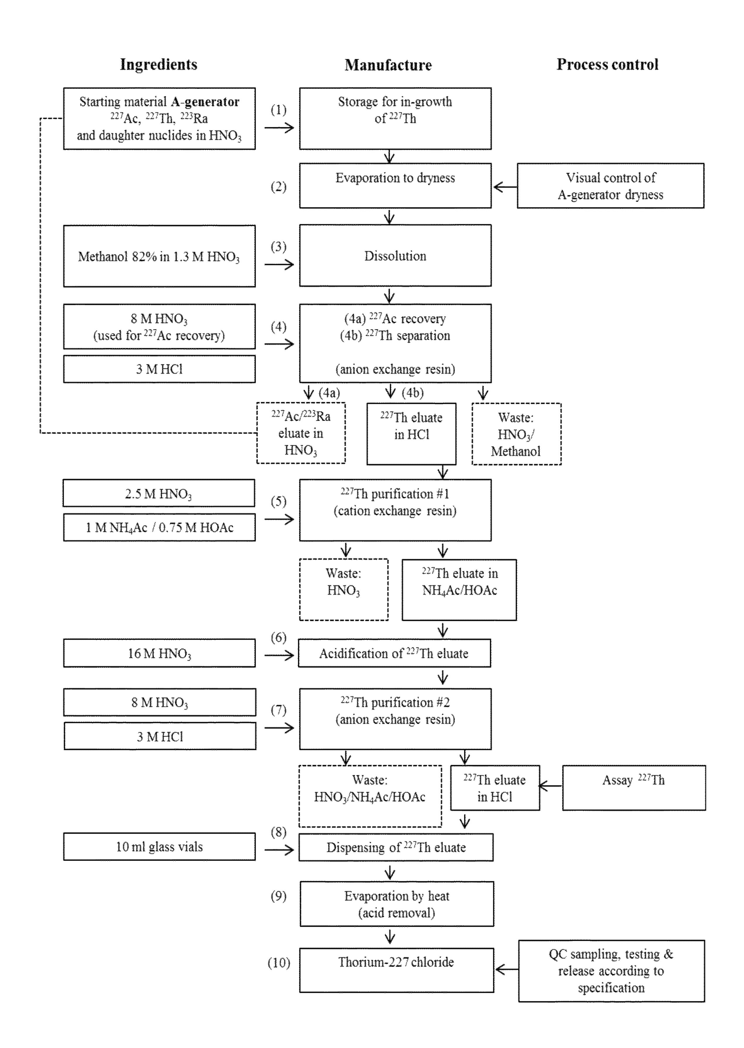
Figure 1 - Manufacturing process and process control
