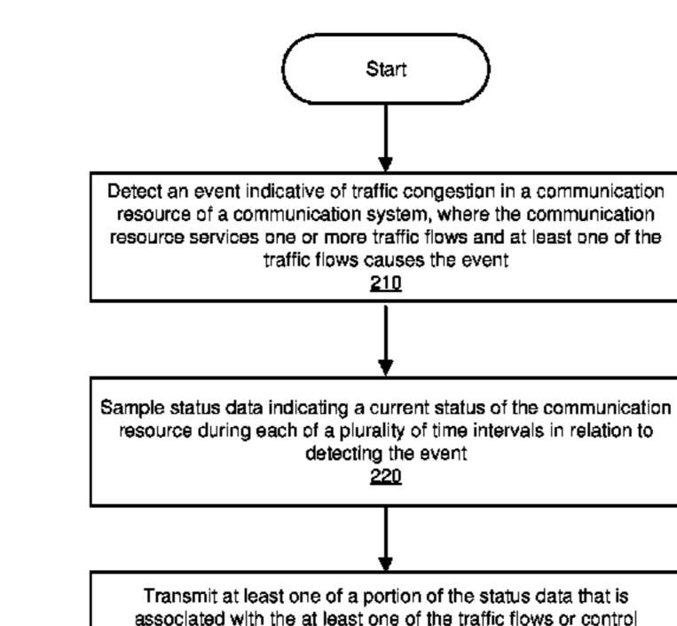
associated with the at least one of the traffic flows or control information for the at least one of the traffic flows to a receiving device external to the communication resource to control the communication system <u> 230</u>
