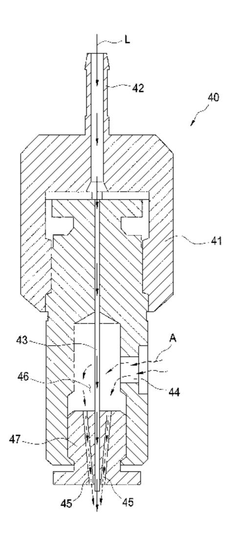
charged from the nozzle part and an aqueous curing agent solution. In the apparatus for immobilizing a microbial cell according to the present disclosure, since the cell-carrier-containing mixed solution is injected through an air spraying nozzle, even when an immobilized carrier solution having a high viscosity is used, a microbial cell immobilized bead having a small size and having a spherical shape, or an almost spherical shape may be mass-produced.
