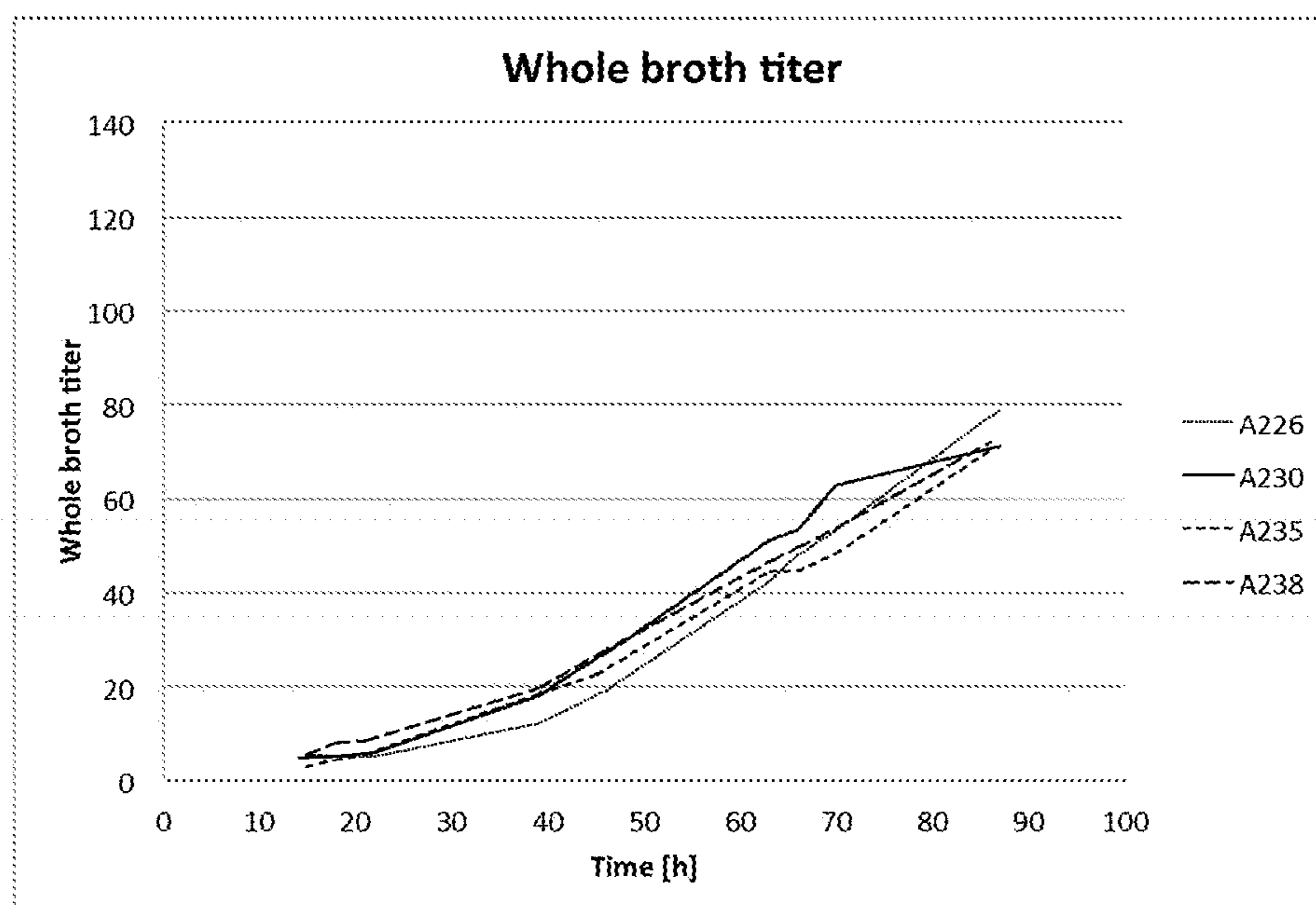
Figure 31: Whole Broth Titer profile for 4 different feed rates indicating product expression for mAb3 antibody Strain B in 20L fermentors
