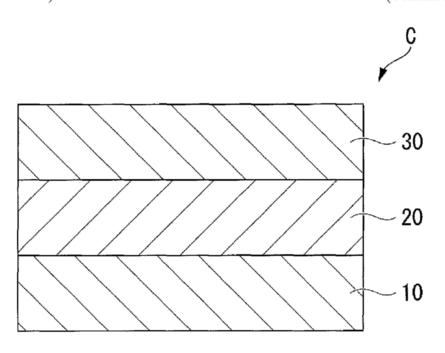
included in the second catalyst layer, in terms of cerium dioxide, is 10-25 g per liter of the fire-resistant three-dimensional structural body.
