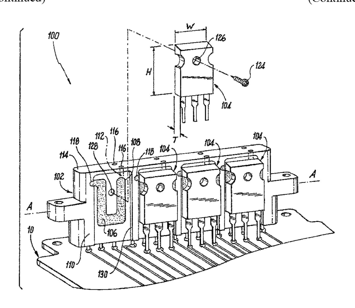
Injecting a bonding agent can include ceasing injection of bonding agent upon appearance of bonding agent in a window opening in fluid communication with the open channel.
