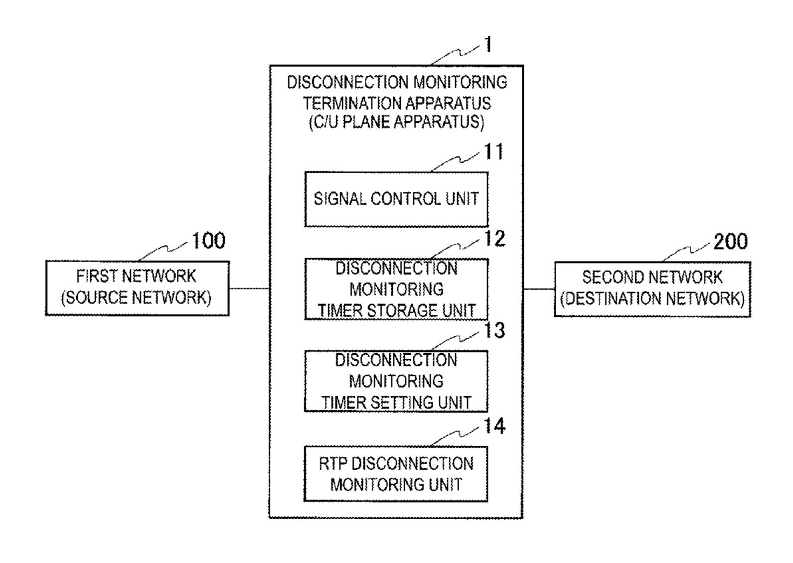
timer of the first network 100, and when detecting the inability to communicate the RTP packets in the second network 200, the disconnection monitoring termination apparatus 1 sends an UPDATE request or a re-INVITE request including an SDP offer in which a direction attribute of "a=recvonly" is set, to the first network 100.
