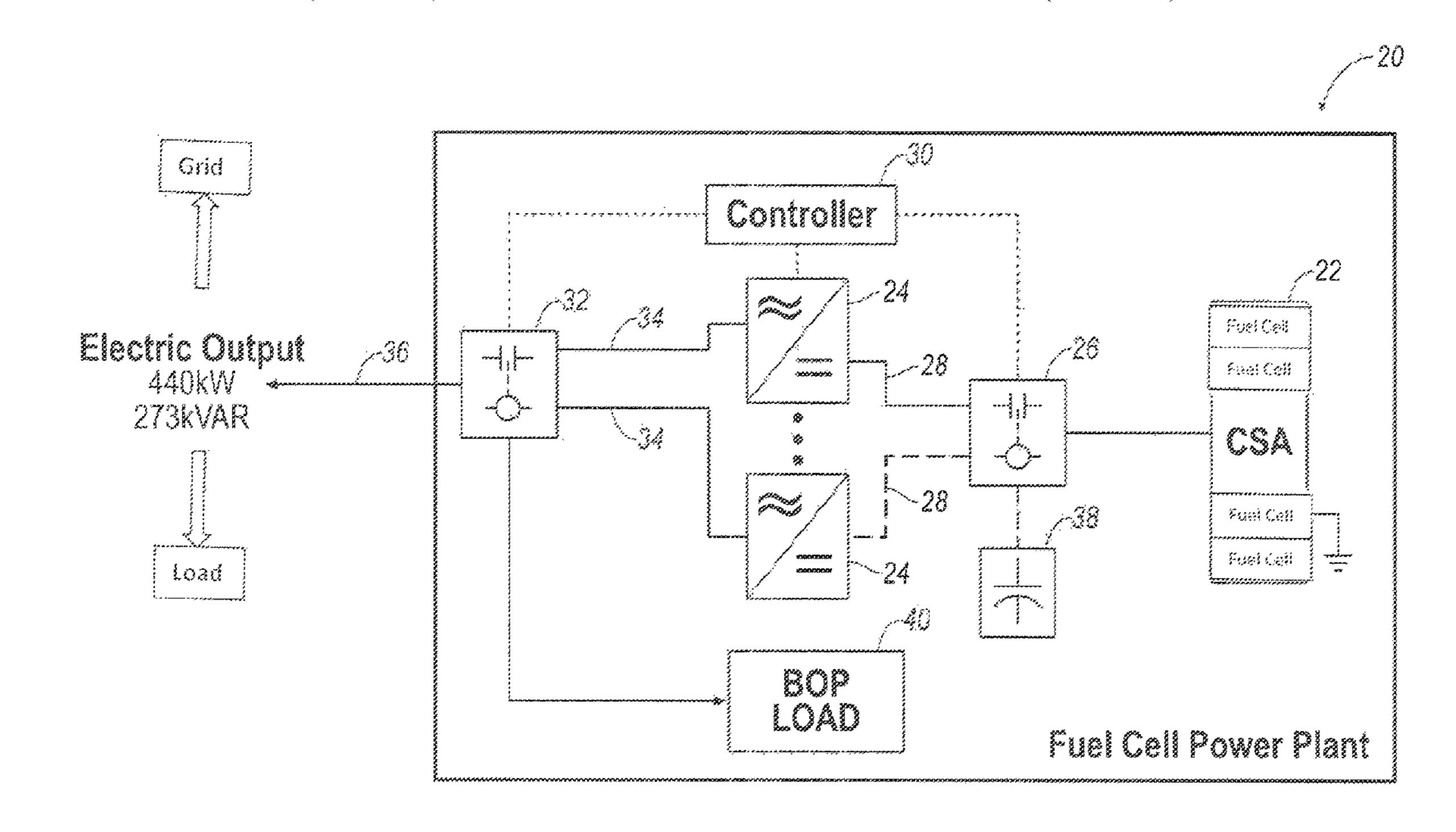
inverters selectively provide reactive power to or receive reactive power from a grid external to the fuel cell power plant in the second mode.
