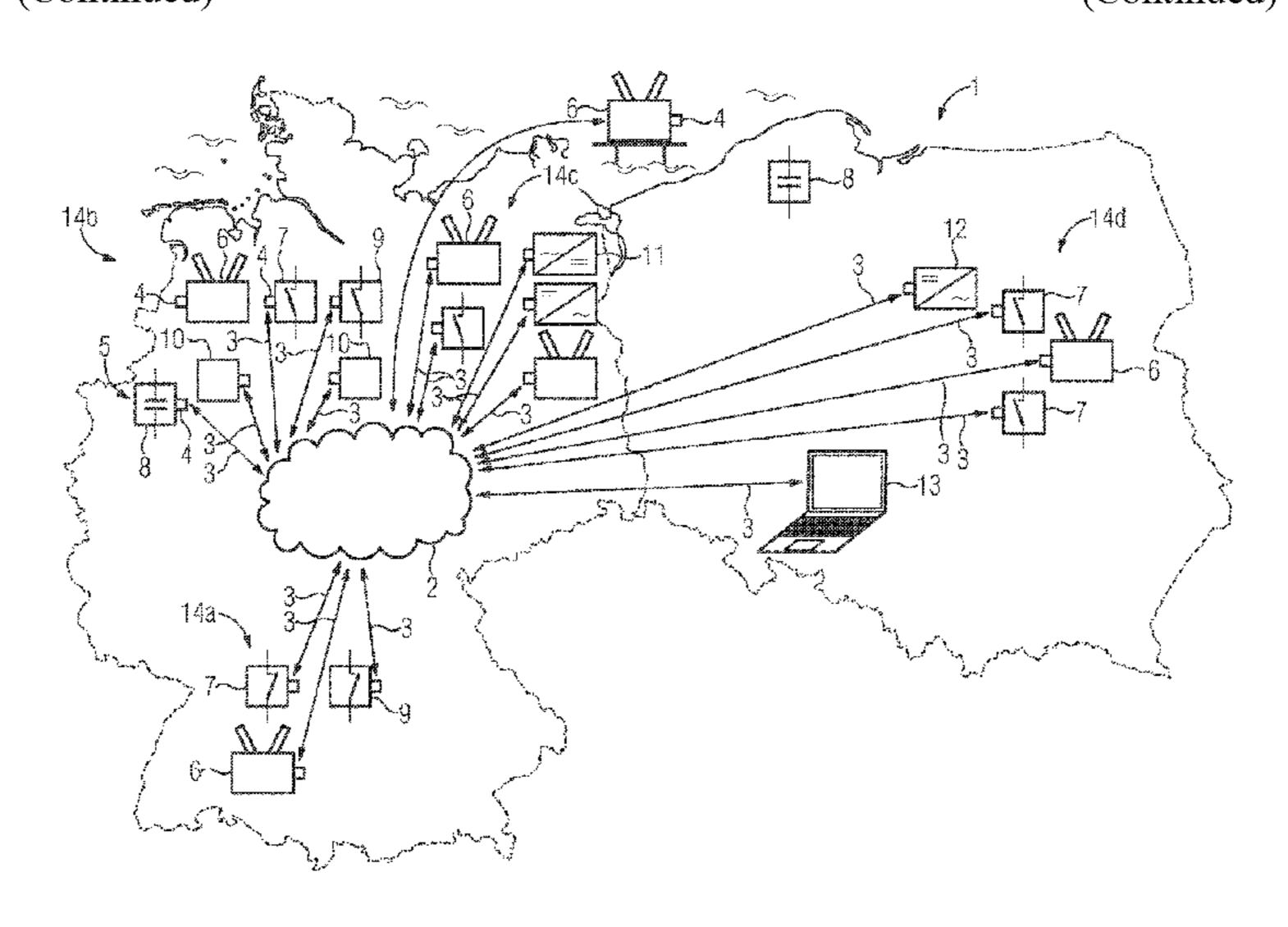
cost-effective analysis of the entire network operating state, the data processing cloud during analysis uses measured values and/or values derived therefrom from at least two selected communication units at different locations.
