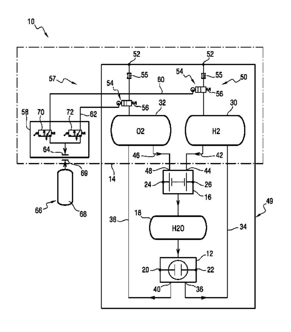
discharge valve, a fluid pipe fluidically connecting the operating station to the discharge valve, the operating station including at least one reversible free connection for connecting to each fluid pipe of a device for supplying the control system with operating fluid.
