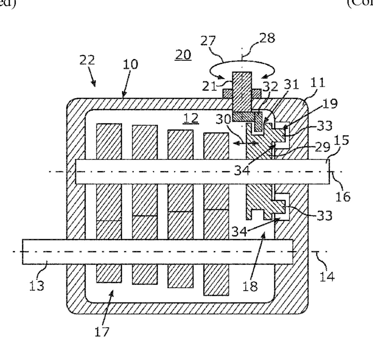
release position in which the at least one locking element releases the shaft for rotation relative to the housing.
