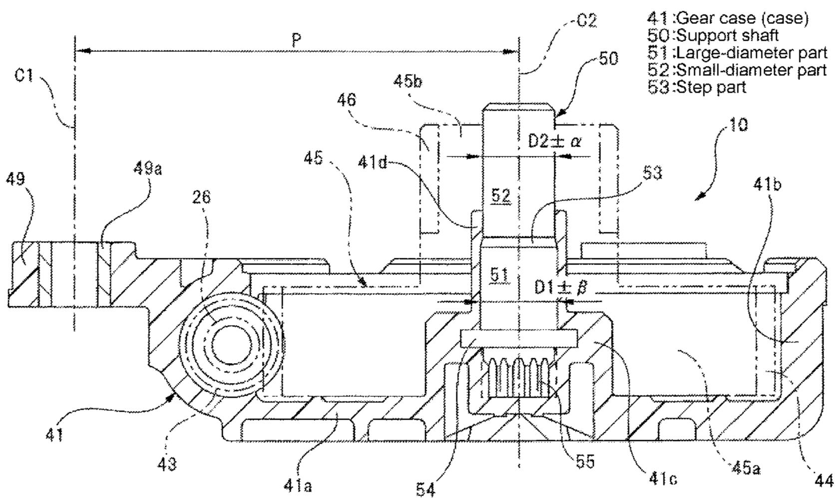
diameter part and the step part are embedded in the gear case, the resistance of the support shaft against pulling from the gear case can be enhanced.
